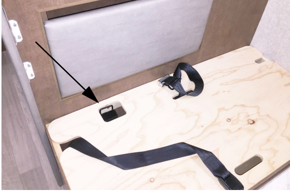
Tether Anchor Loop (Located beneath the forward facing dinette seat back cushion)
