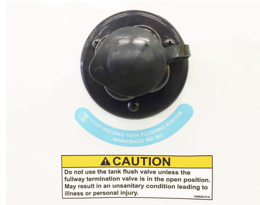
Black Waste Tank Flush Inlet (Located on backwall or left sidewall, depending on model) -Typical View
