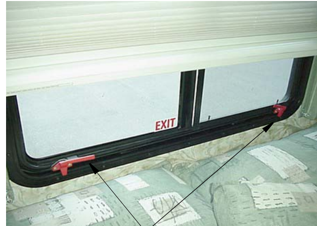
Escape Window - Lift latch handles upward to open
