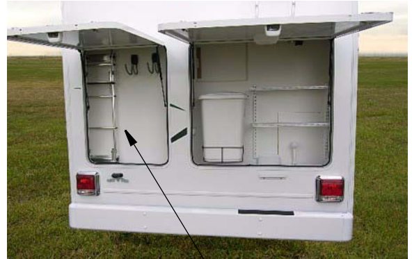
Roof Ladder Extension Storage
