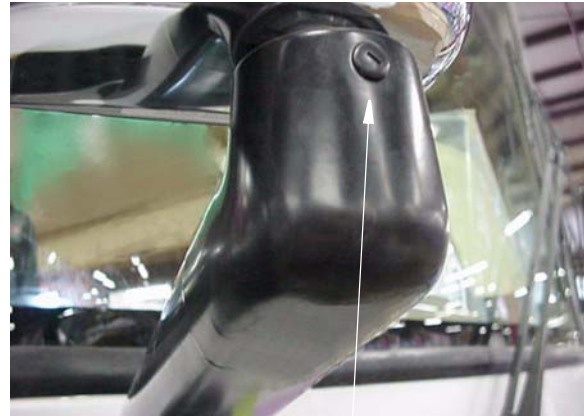
Mirror Pivot Lock Unscrew protective cap and loosen Allen head set screw
