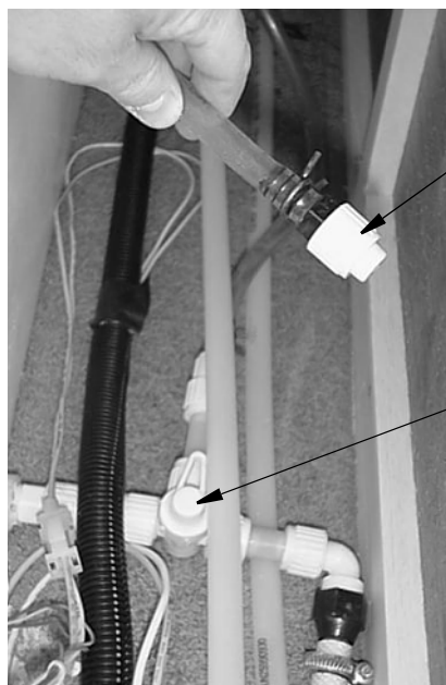
Winterization Valve (See Water Drain Valve Location chart for location on your coach)
