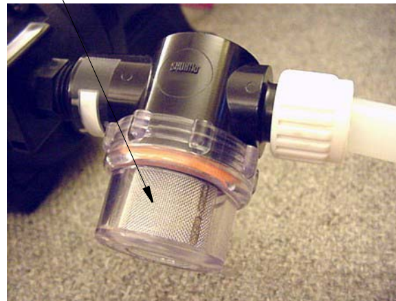
Water Pump Strainer
