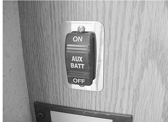
Aux. Batt. Switch (Near entrance door)
