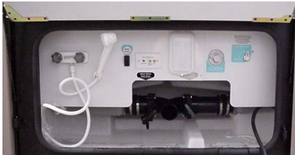
Water Service Center
