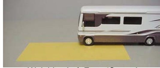
Weighing Left Front 'Corner'
