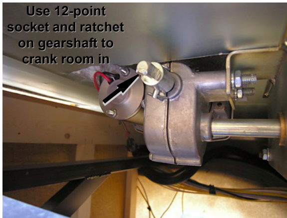
Model 29H Rear Slideout Room Motor/Gear Assembly (view from access panel at foot of bed)
