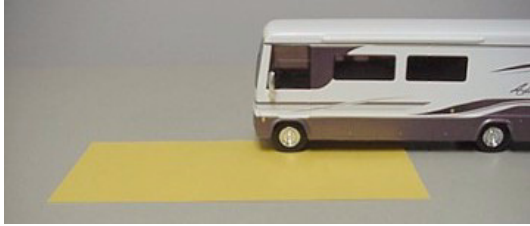
Weighing Left Front 'Corner'
