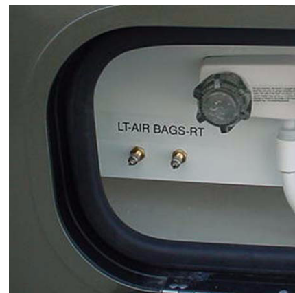
Rear Air Helper Spring Valves (located in water service center compartment)
