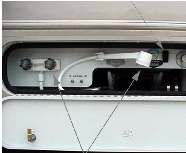
Exterior Shower/Wash Station (Typical)
