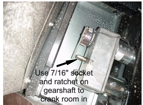
Model 23D Front Slideout Room Motor/Gear Assembly (view from ground)
