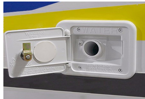
Water Tank Gravity Fill
