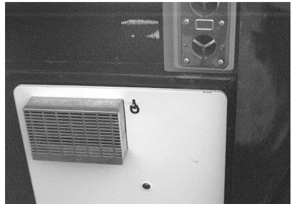
Water Heater Service Access Panel
