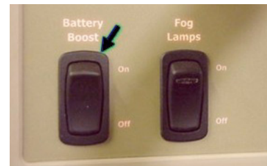
Battery Boost Switch
