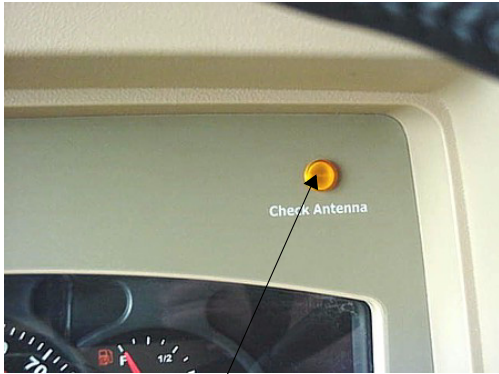
"Check Antenna" Light
