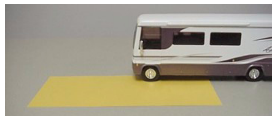
Weighing Left Front 'Corner'
