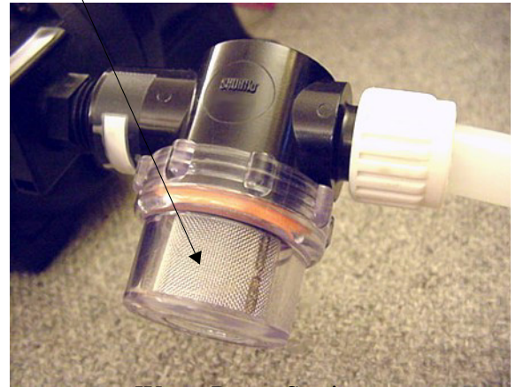
Water Pump Strainer
