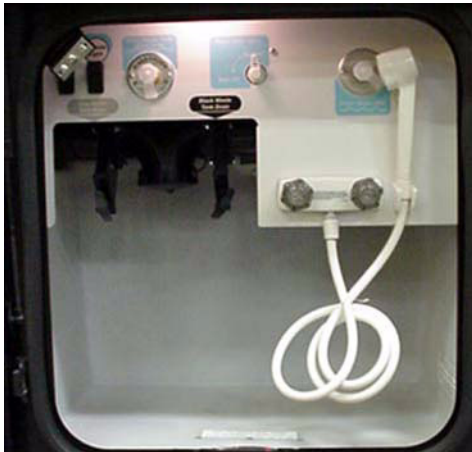
Water Service Center
