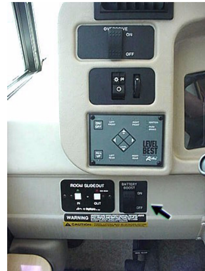
Battery Boost Switch
