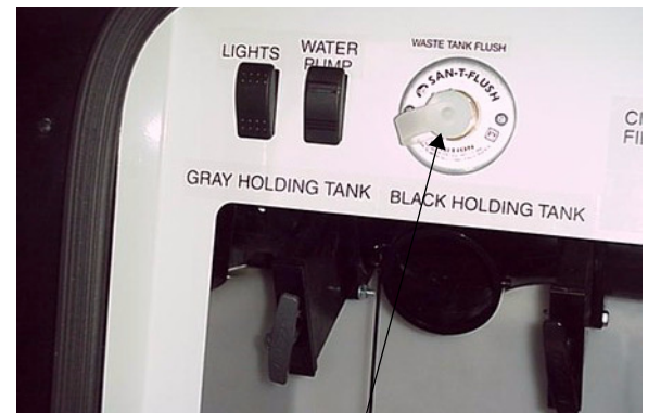
Waste Tank Flush
