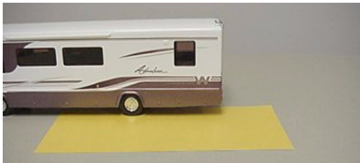
Weighing Left Rear 'Corner'
