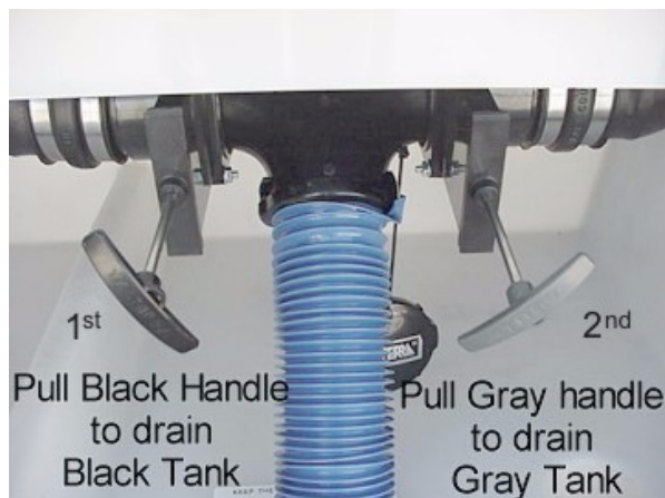
Holding Tank Valves (Typical)
