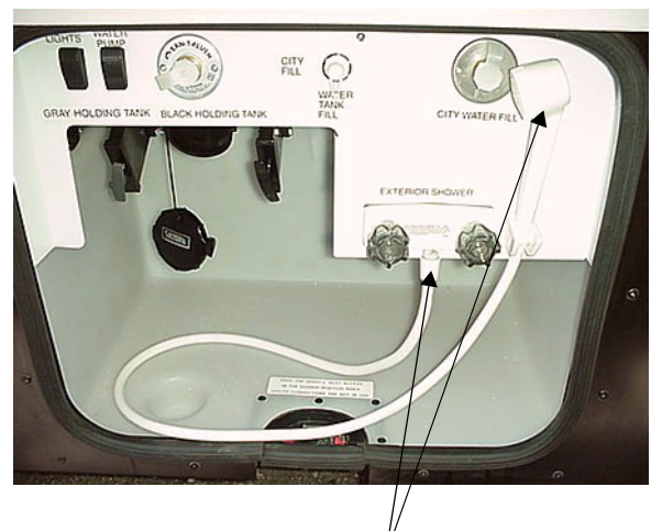
Exterior Shower/Wash Station
