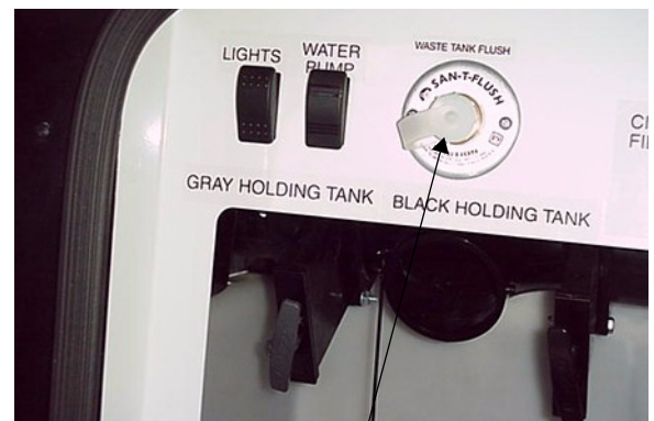
Waste Tank Flush
