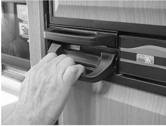
Push door handle downward and pull to open refrigerator. Lift freezer handle to open.
