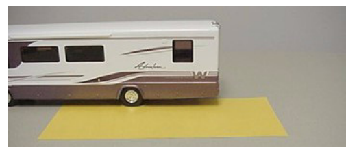
Weighing Left Rear 'Corner'
