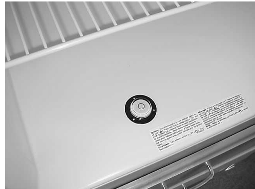
Place bubble level in bottom of refrigerator
