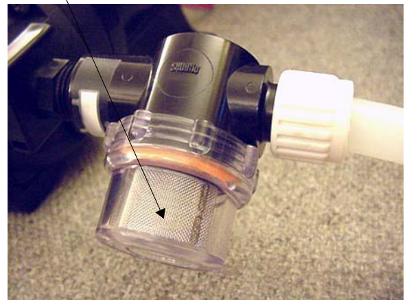
Water Pump Filter
