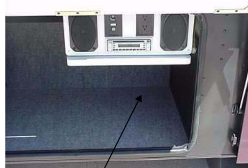
Entertainment Center (In right front cargo compartment)
