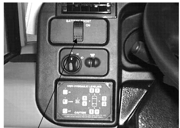
Battery Boost Switch
