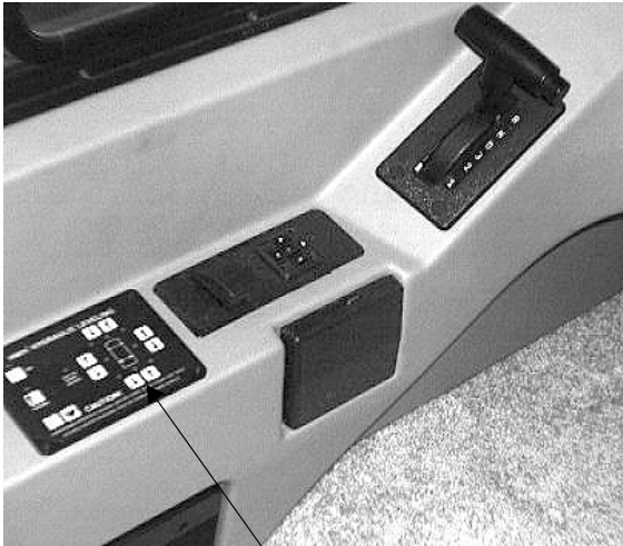
Leveling System Control Panel
