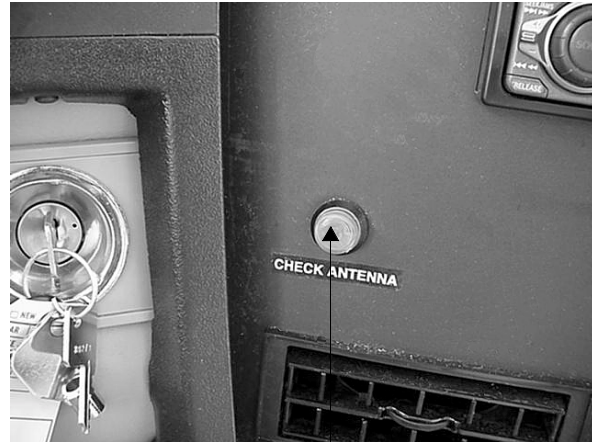
"Check Antenna" Light
