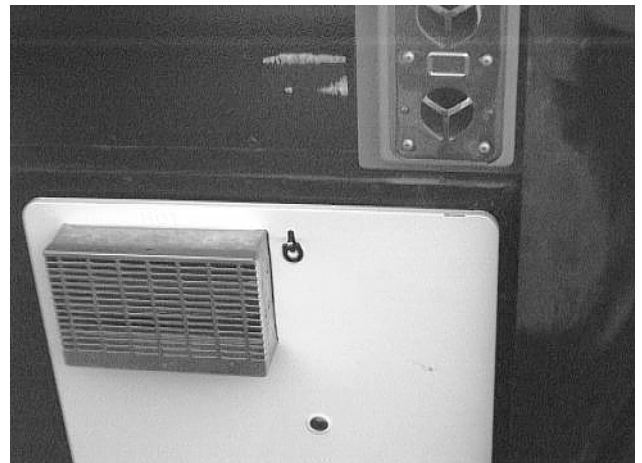
Water Heater Service Access Panel
