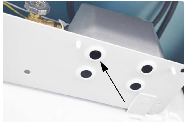
Look up inside hole on underside of regulator housing to see vent screen.
