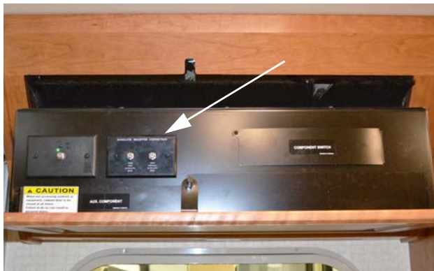
Interior Connection for Satellite Dish -Typical View
