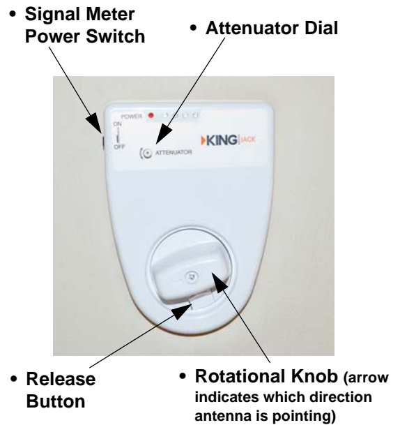
Digital Antenna Signal Meter (Located on ceiling)
