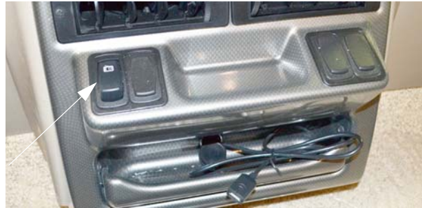
Radio Power Switch (Located on lower dash area)
