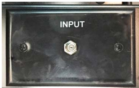
Cable TV Connection (Located in water service center or utility compartment, depending on model)
