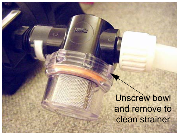
Water Pump Strainer -Typical View
