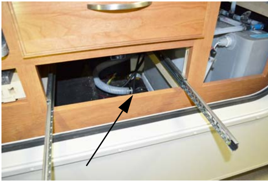
Waste Pump (Located inside passenger side rear compartment, remove bottom drawer below sink to access) -If Equipped
