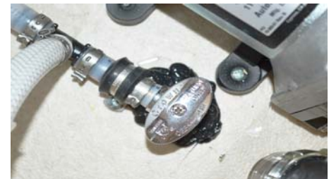
OFF ON Water Tank Drain Valve (Typical)
