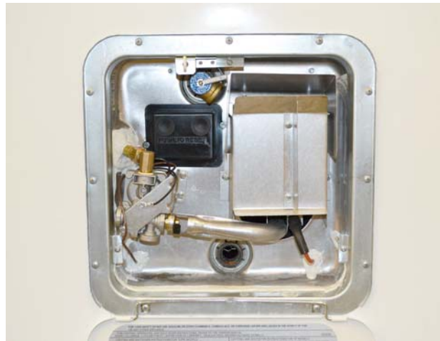
Water Heater Exterior Service Access
