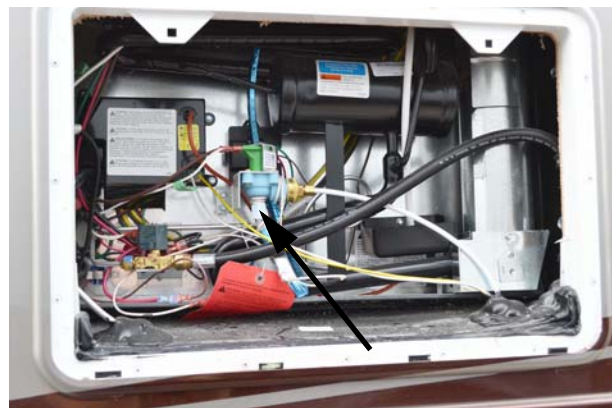
Ice Maker Water Supply Connection -Typical View
