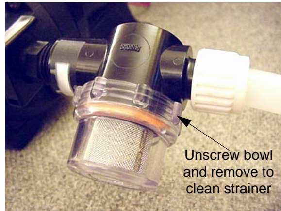
Water Pump Strainer -Typical View
