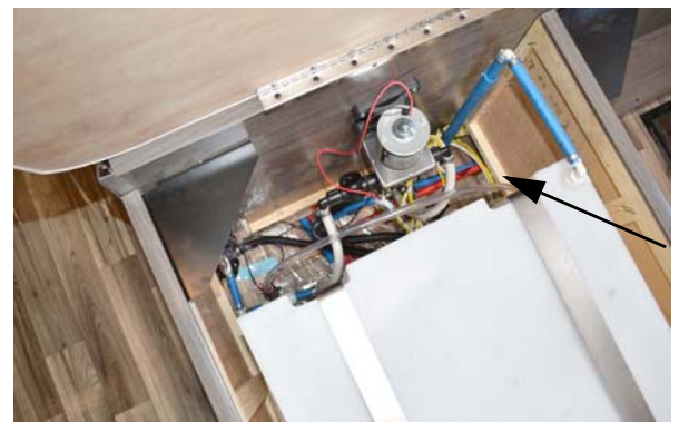
Water Pump (Located beneath bed - extend rear bed slideout, remove mattress from bed, and lift hinged bed board to access) *Model 26A
