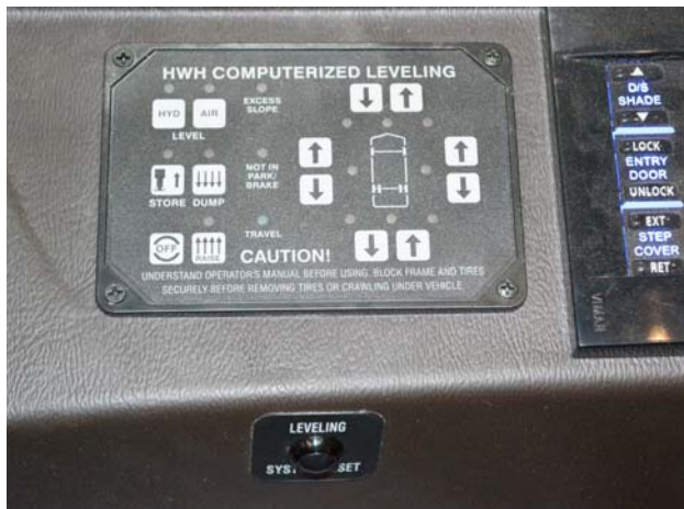
Air and Hydraulic Leveling System Control Pad and Leveling System Reset Switch
