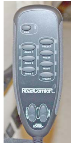
Cab Seat Massage Remote Control (Located on inboard side of driver and co-pilot seats)
