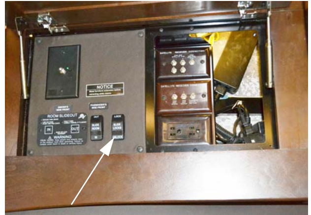
Slideout Room Travel Lock (Your model may be equipped with one or more types) -Typical View
