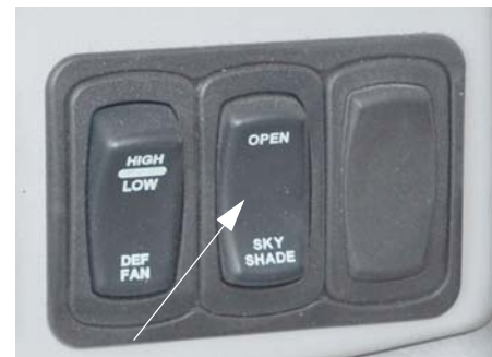
Skylight Shade Control Switch (Located on dash)
