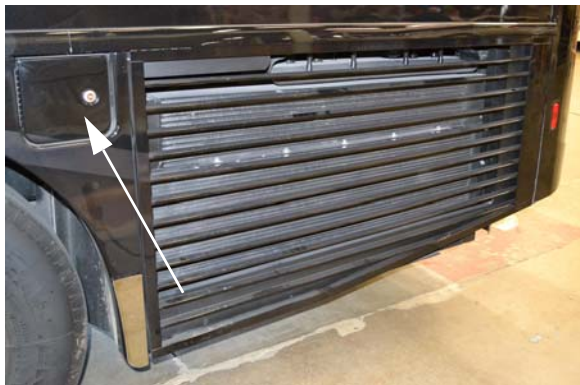
Diesel Exhaust Fluid Remote Fill *with Side Radiator (Located on driver side forward of side radiator) -Typical View
