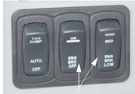
Engine Brake Activation Switches (Located on driver side trim panel) -Typical View
