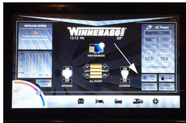
Generator Switch (Located on touch tablet "Home" screen) Push and Hold for 10 seconds to turn on. • White text indicates ON.
