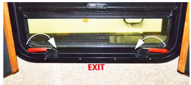
Escape Window (Lift both red safety latch handles UP and push window OUT) -Typical View
