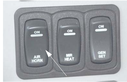
Air Horn Switch (Located on dash or driver side trim panel) -Typical View
