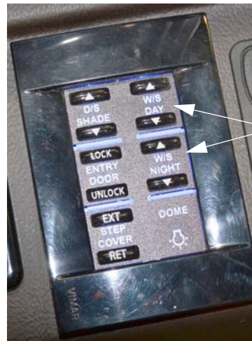
12-Volt Front Drop-Down Solar/Night Shade Switches (Located on driver side trim panel) -Typical View
