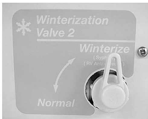
Winterization Valve 2 (Located near water pump - second compartment on driver side of coach)
