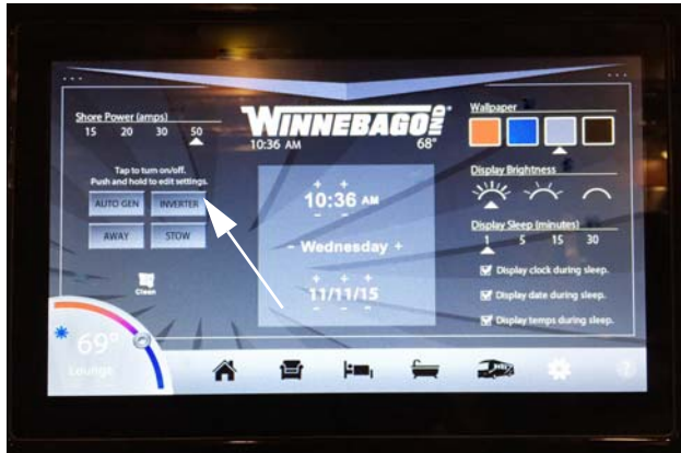
Inverter Power Switch (Located on touch tablet “Utilities” screen) Tap “Inverter” to turn on/off. • White text indicates ON. • Black text indicates OFF.
