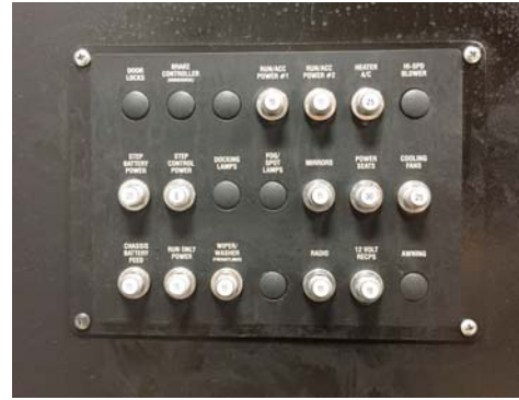
Automotive Circuit Breakers (push to reset) • Breakers are labeled for components equipped
