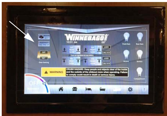
Hydronic Heating System Interior Control Switches
