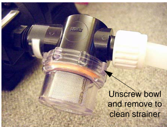
Water Pump Strainer -Typical View
