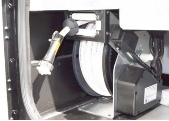
Water Hose Reel (Located in the water service center) -Typical installation shown
