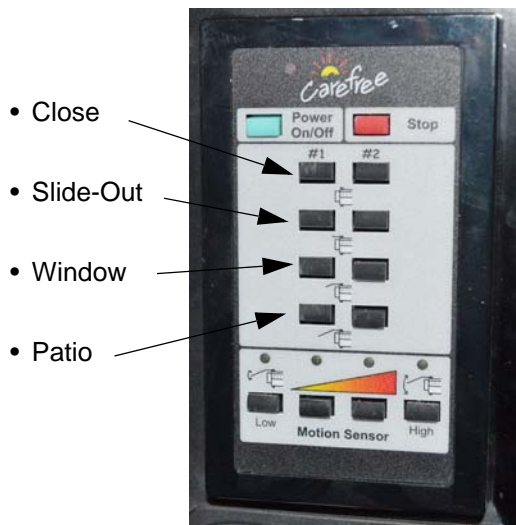
Power Awning Control Switches (Located near the entrance door) -Typical View
