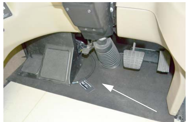
CB Power Wires -Typical View
