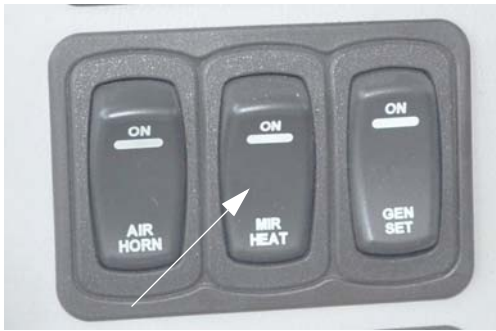
Mirror Heater Switch (Located on dash) -Typical View
