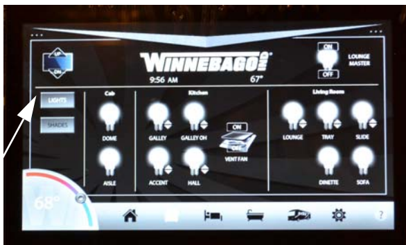
Power Roof Ventilator Switch (Located on touch tablet “Lounge” screen) -If Equipped
