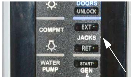
Auto Level Remote Switch (Located near entrance door and/or inside exterior service center) -Typical View
