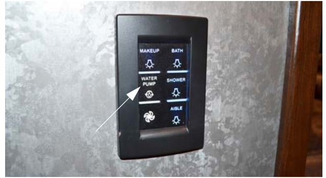
Water Pump Switch (Located in all bath areas) -Typical View The switch will illuminate blue when the switch is on. White illumination indicates the switch is off.
