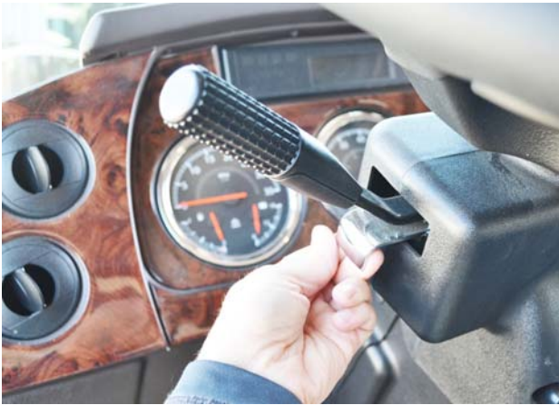
Hazard Warning Flashers (Typical View - your coach may differ depending on model)
