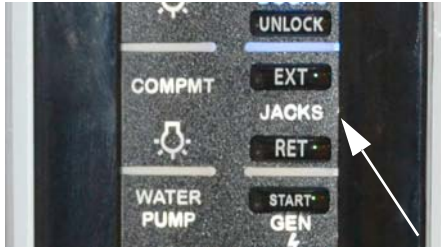
Auto Level Remote Switch (Located near entrance door and/or inside exterior service center) -Typical View
