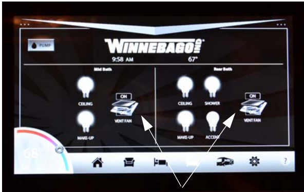
Power Roof Ventilator Switch (Located on touch tablet “Bath” screen) -If Equipped
