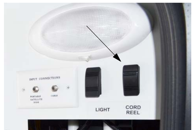
Power Cord Reel Switch (Located near the power cord reel) -Typical View
