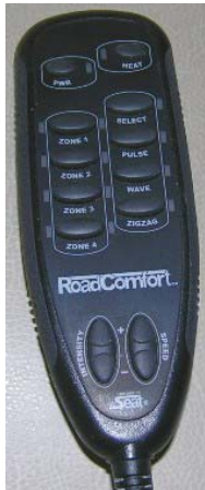
Luxury Cab Seat Remote Control (Located on inboard side of driver and co-pilot seats)
