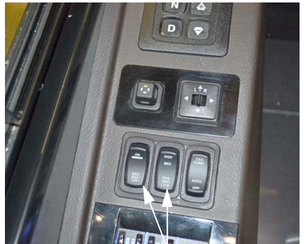
Engine Brake Activation Switches (Located on driver side trim panel) -Typical View
