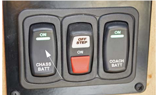
Chassis Battery Disconnect Switch (Located near entrance door) -Typical View
