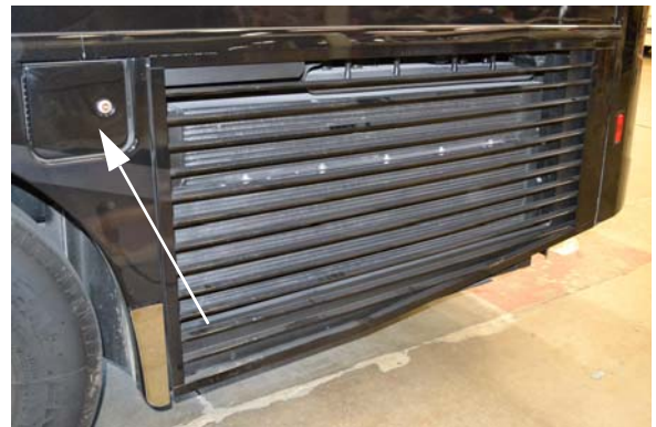
Diesel Exhaust Fluid Remote Fill *with Side Radiator (Located on driver side forward of side radiator) -Typical View
