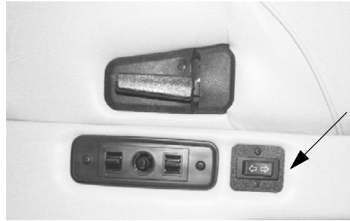
Power Footrest Switch (Located on inboard side of co-pilot seat) -Typical View
