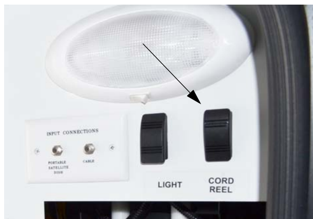
Power Cord Reel Switch (Located near the power cord reel) -Typical View
