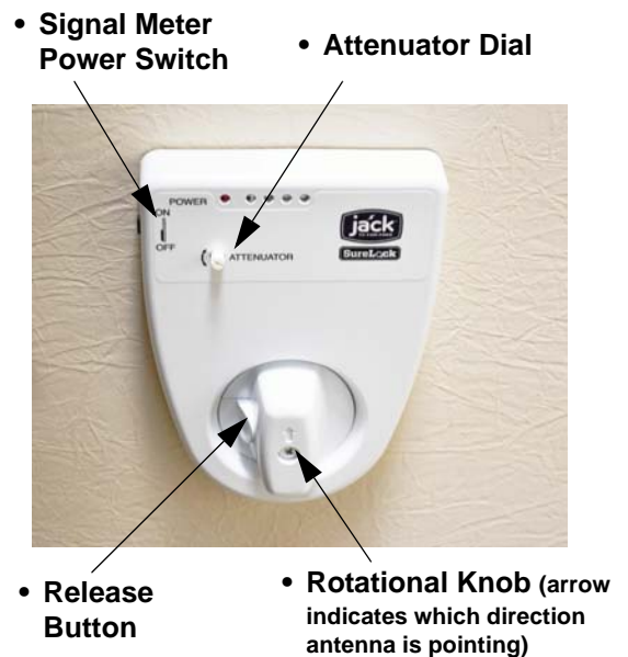
Digital Antenna Signal Meter (Located on ceiling)
