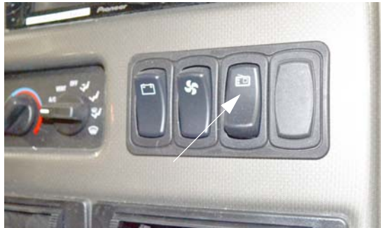
Radio Power Switch (Located on lower dash area)
