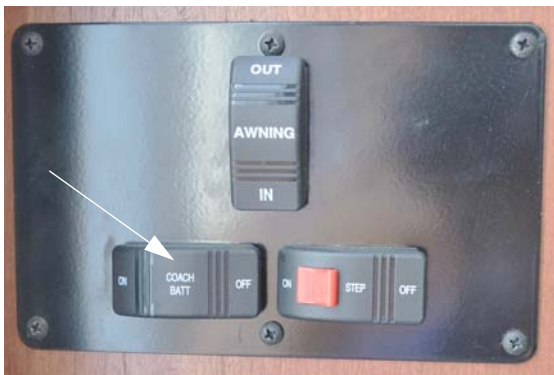
House/Coach Battery Disconnect Switch (Located near entrance door)
