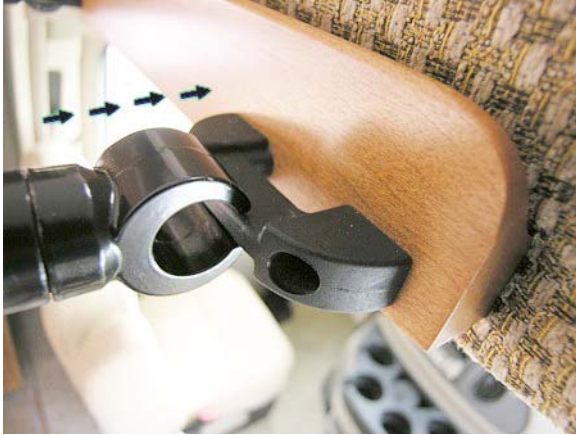
Attaching Bunk Ladder
