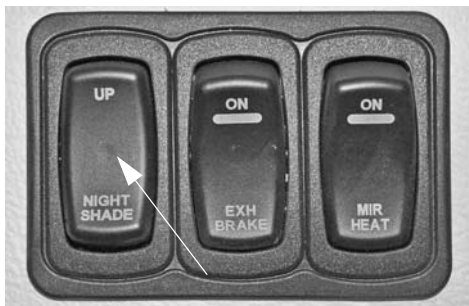
12-Volt Front Drop-Down Night Shade Switch (Located on driver side trim panel) -Typical View
