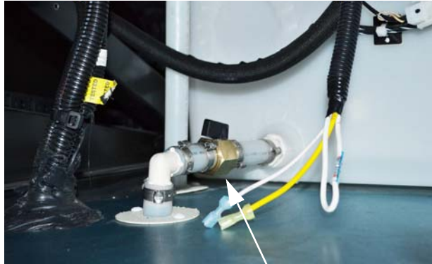
Water Tank Drain Valve (Located in second driver side compartment) *Model 34T shown
