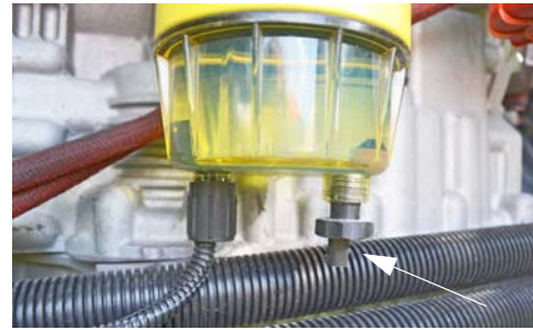
Fuel/Water Separator Drain Valve (Located on bottom end of separator) -Typical View
