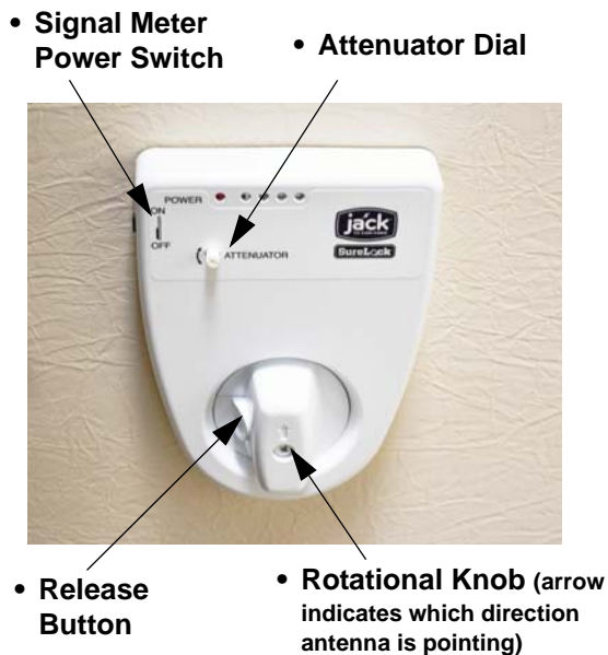
Digital Antenna Signal Meter (Located on ceiling)
