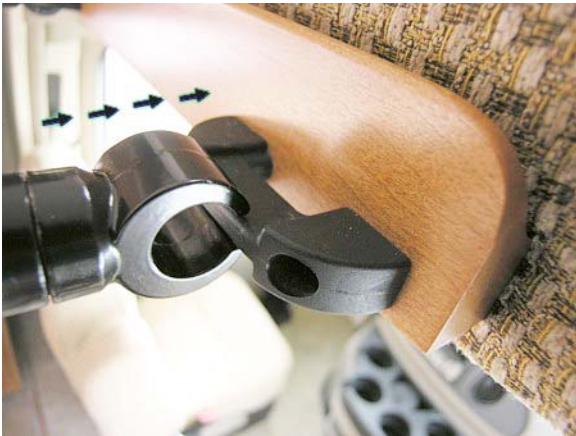
Attaching Bunk Ladder
