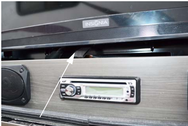
Pull black strap straight down to release the TV from the mounting bracket.
