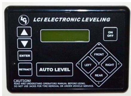
Leveling System Control Panel (Located on dash)
