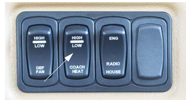
Coach Heat Switch -Typical View
