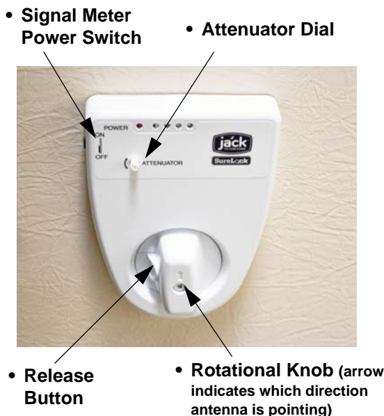
Digital Antenna Signal Meter (Located on ceiling)
