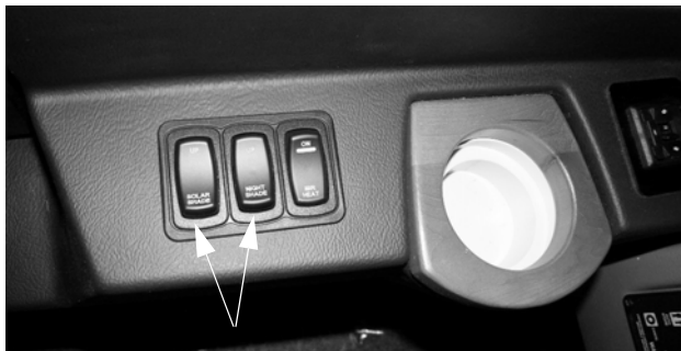
12-Volt Front Drop-Down Solar/ Night Shade Switches -Typical View
