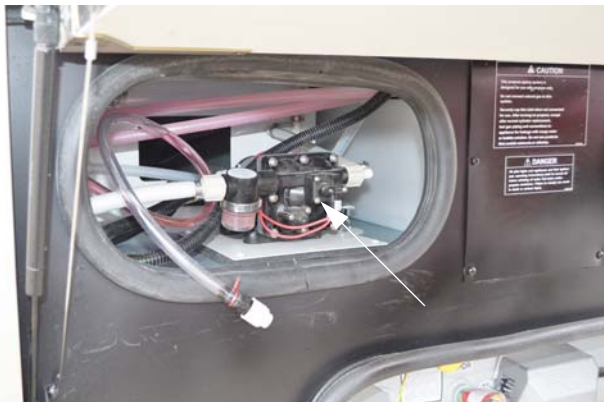
Water Pump (Located in compartment behind rear passenger side tire) * Model 37F shown
