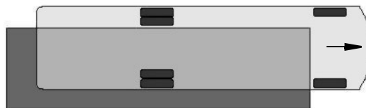
Weighing Right Rear Corner
