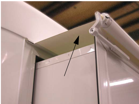
Slideout Cover-Awning -Typical View
