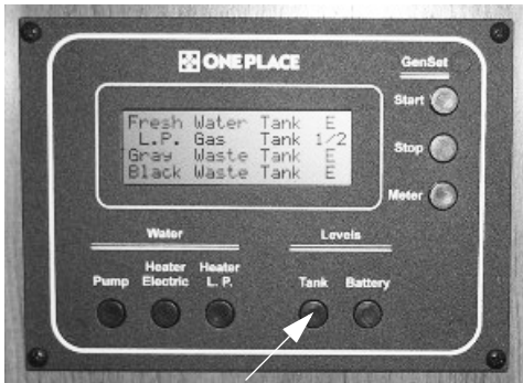
Tank Levels Switch
