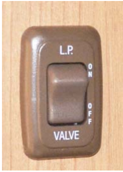
LP Tank Valve Switch
