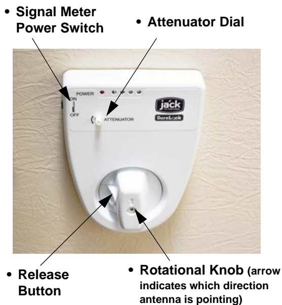
Digital Antenna Signal Meter (Located on ceiling)
