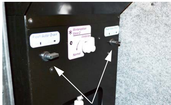
Waterline Drain Valves (Located in the third passenger side compartment) -Typical View
