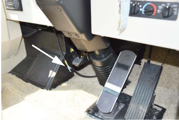
CB Power Wires -Typical View
