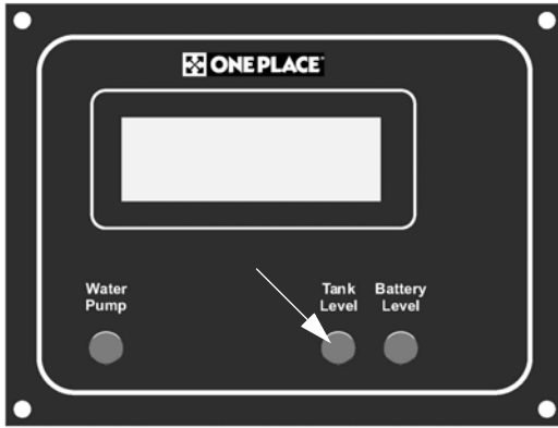
Tank Level Switch
