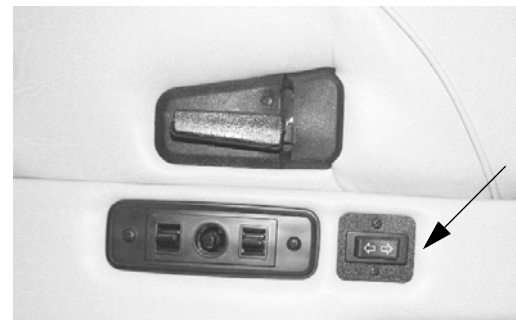
Power Footrest Switch (Located on inboard side of co-pilot seat) -Typical View
