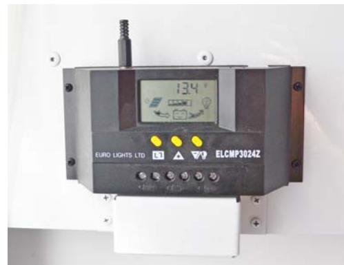
Solar Charge Controller (Located in utility compartment)
