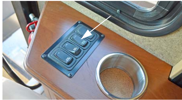
Power Door Locks - Entry Door (Located on passenger side trim panel) -Typical View
