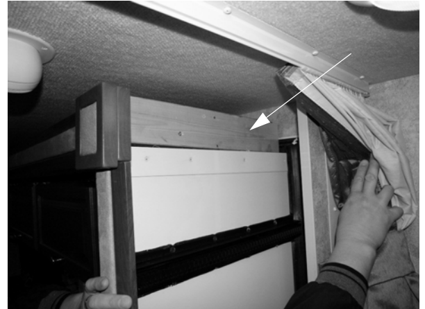
Slideout Travel Support -Typical installation shown
