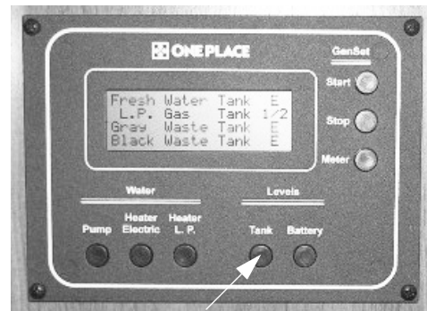
Tank Levels Switch
