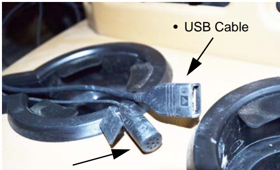
Bluetooth Microphone and USB Cable (Located on the dash beverage tray) -Typical View (if equipped)
