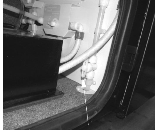
Waterline Drain Valve - Typical Installation
