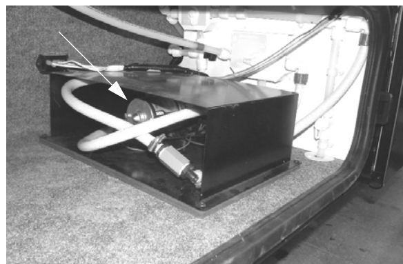
Water Pump (Located in compartment behind entrance door) * Models 32H and 35P shown -Typical Installation
