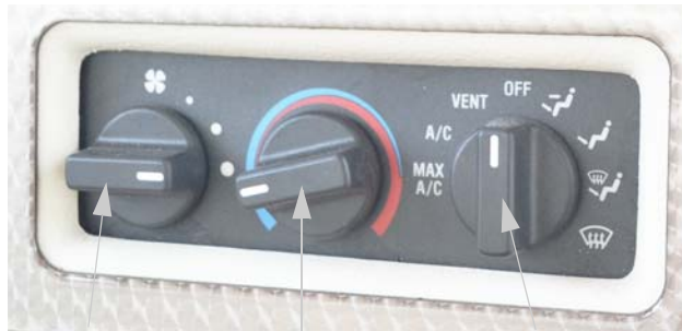
Blower Control Temp Control Mode Selector
