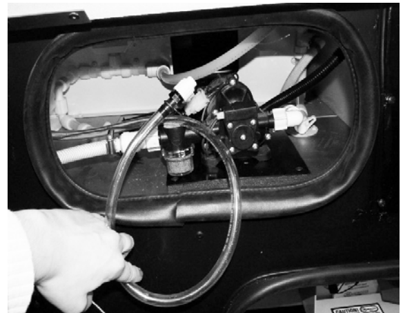
RV Antifreeze Siphon Tube (See the “Water System Drain Valve Locations” chart at the end of this section for location on your coach) -Typical View
