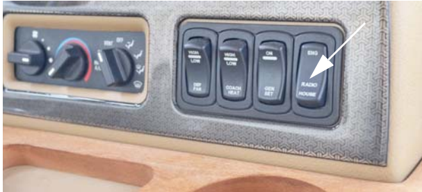
Radio Power Switch (Located on dash)
