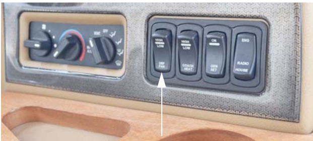
Defrost Fan Switch (Located on dash) -Typical View
