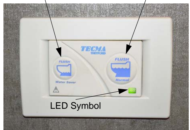
Wall Switch/Controller (Located on wall near toilet)
