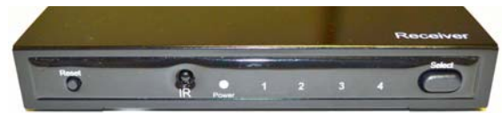
Secondary Source Selector (Located near each TV)
