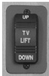
Buffet TV Power Lift/Lower Control Switch (Located on galley end near buffet)
