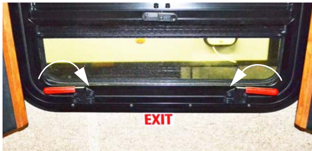
Escape Window (Lift both red safety latch handles UP and push window OUT) -Typical View
