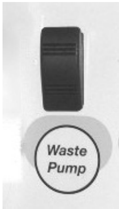
Waste Pump Switch (Located in driver side compartment) -Typical View
