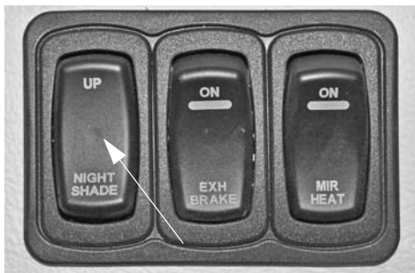
12-Volt Front Drop-Down Night Shade Switch (Located on driver side trim panel) -Typical View
