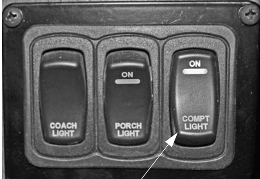
Compartment Lights Switch (Located near entrance door) -Typical View
