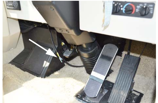
CB Power Wires -Typical View
