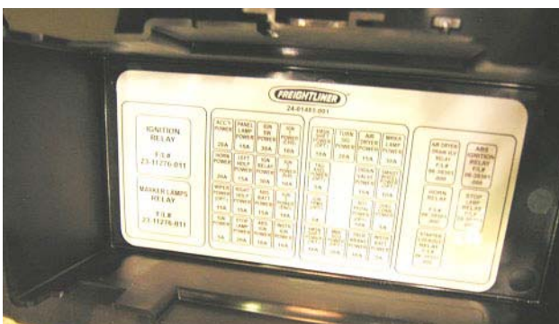
Fuse Diagram (inside of cover)
