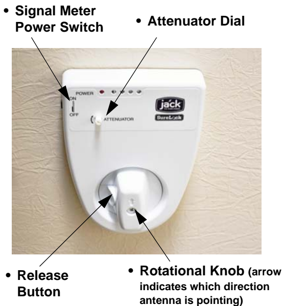
Digital Antenna Signal Meter (Located on ceiling)
