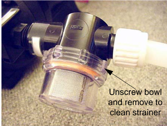
Water Pump Strainer -Typical View
