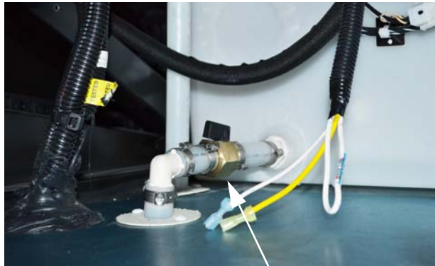
Water Tank Drain Valve (Located in second driver side compartment) -Typical installation shown
