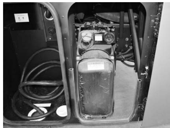
Diesel Exhaust Fluid Fill Tank (Located in passenger or driver side compartment behind rear wheel, depending on model) -Typical View
