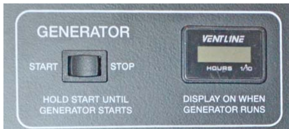
Generator Switch and Hourmeter on monitor panel -Typical View
