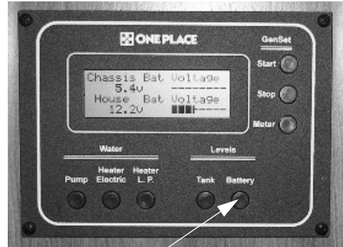
Battery Levels Switch
