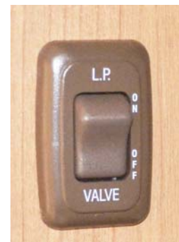
LP Tank Valve Switch
