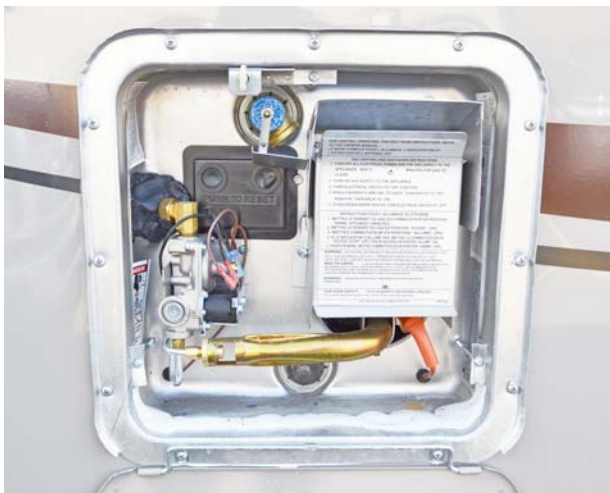
Water Heater Exterior Service Access
