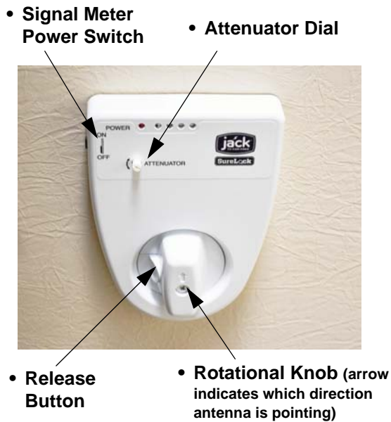
Digital Antenna Signal Meter (Located on ceiling)
