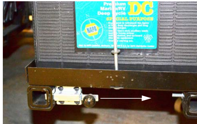
Pull locking device straight out (toward front end of coach) to release slide tray
