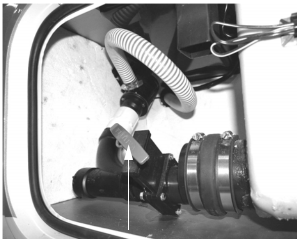
Gray Waste Tank Drain Valve (Located in driver side compartment behind rear wheel)
