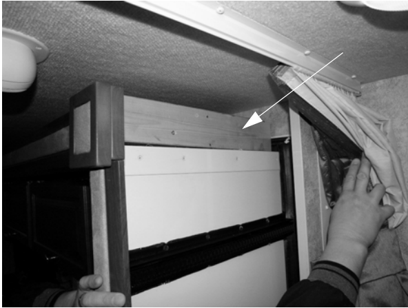
Slideout Travel Support -Typical installation shown
