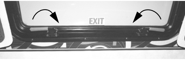
Escape Window (Lift both red safety latch handles UP and push window OUT) -Typical View
