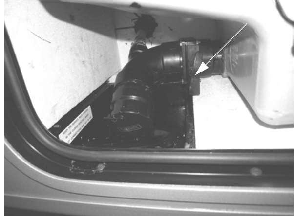
Black Waste Tank Drain Valve (Located in driver side compartment ahead of rear wheel)
