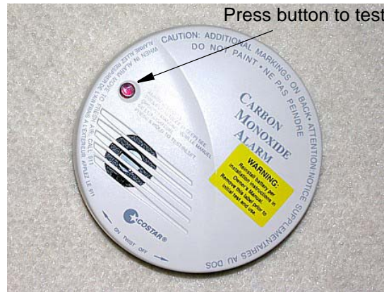
Carbon Monoxide Alarm
