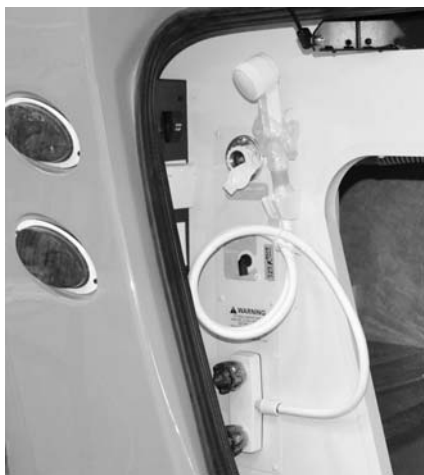
Exterior Shower/Wash Station (Located in backwall exterior service center)
