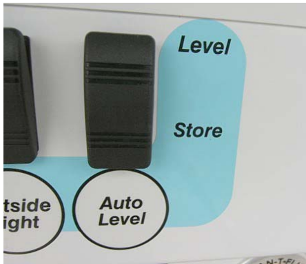
Auto Level Remote Switch (Located in exterior service center) -Typical View
