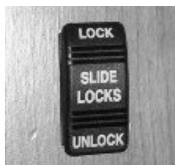
Slideout Room Travel Lock (Your coach may be equipped with one or more types) -Typical View
