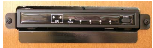
Secondary Source Selector (Located near each TV)
