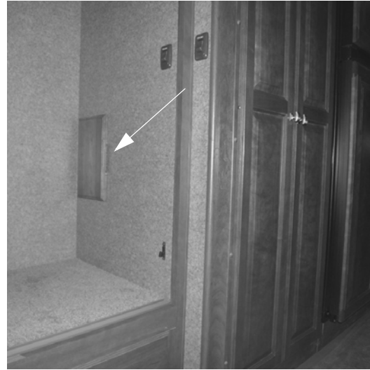
Water Supply Faucets (Located behind access door in wardrobe) * Model 37F shown
