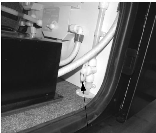
Waterline Drain Valve - Typical Installation
