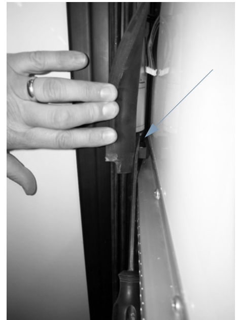
Slideout Motor (Located behind slideout wipe seal) • Use a screwdriver to push slideout motor UP (disengage).
