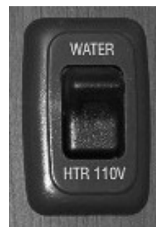
Electric Water Heater Switch (Located near monitor panel)
