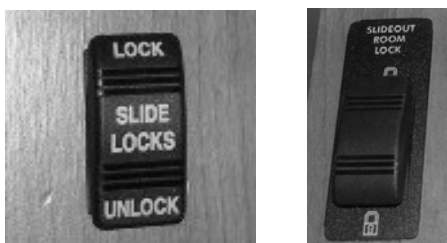
Slideout Room Travel Locks (Your model may be equipped with one or more types) -Typical View
