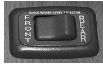
Black Waste Tank Selector Switch (Located near monitor panel) -Typical View
