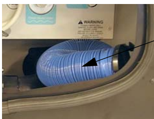
Sewage Drain Hose -Typical View
