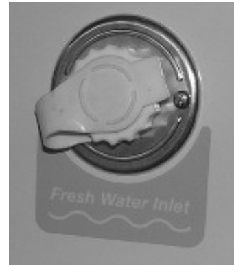
Fresh (City) Water Connection (Fresh Water Inlet)
