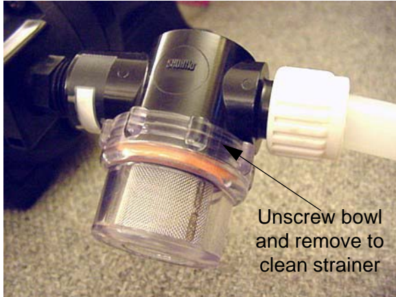
Water Pump Strainer -Typical View
