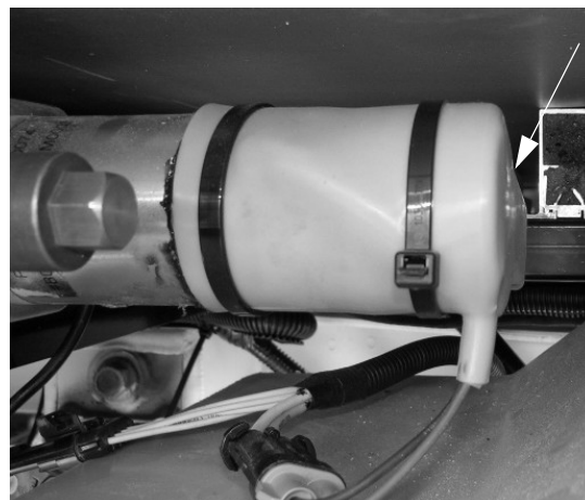
Electric Brake Lever (Located on back side of motor/gear assembly) -Typical View
