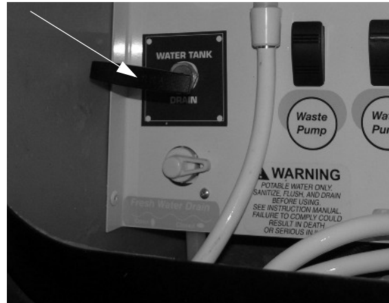
Water Tank Drain Valve (Located in water service center) -Typical View
