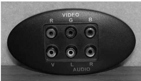
Audio Video Connection Plate -Typical View
