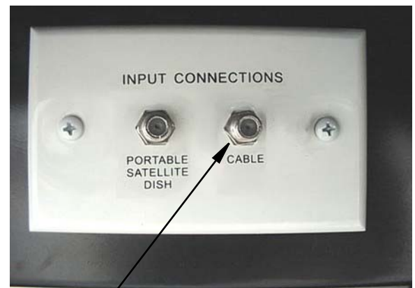
Cable TV Input Hook-Up (Located in Utility Compartment or Shoreline Compartment - depending on model)
