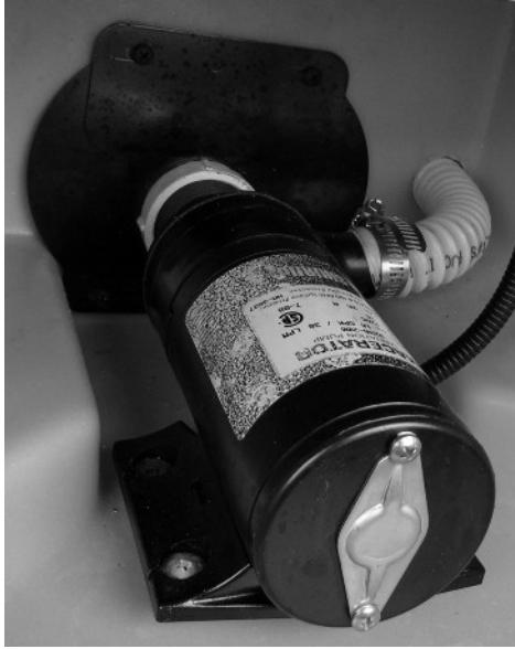
Waste Pump (Located behind removable panel in water service center) -Typical View
