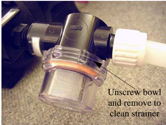
Water Pump Strainer -Typical View
