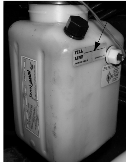
Hydraulic Oil Reservoir -Typical View
