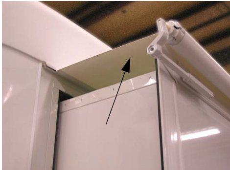
Slideout Cover-Awning -Typical View
