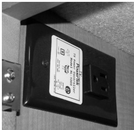
Front TV Ignition Switch Interlock -Typical View
