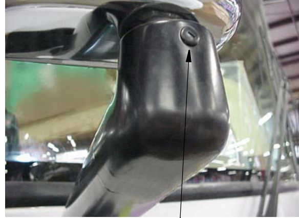
Mirror Pivot Lock Unscrew protective cap and loosen Allen head set screw
