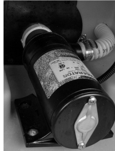
Waste Pump (Located beneath coach) -Typical View
