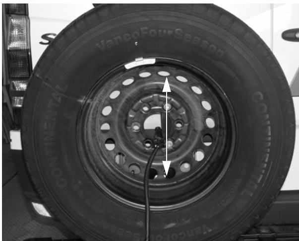
Correct Spare Tire Mounting Locations
