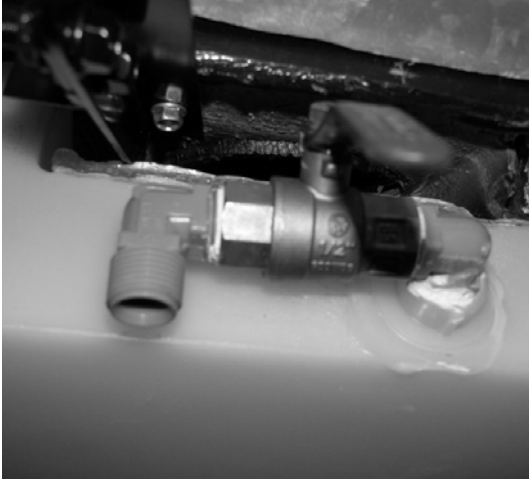
Fresh Water Drain Valve
