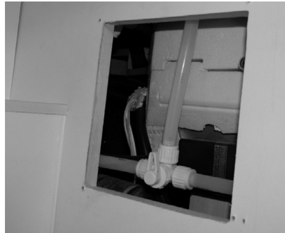
Waterline Drain Valve (Located behind removable panel under rear dinette - open rear doors to access) -Model 144U Shown
