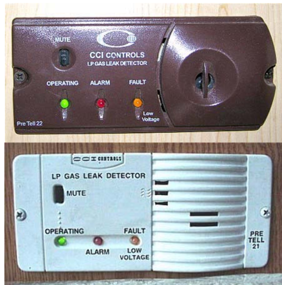
Propane Gas Leak Detectors (Typical)
