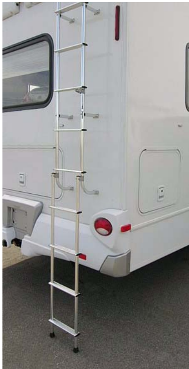
Pull pin to lower ladder extension
