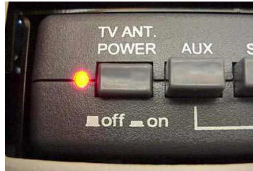
TV Signal Amplifier Switch on Video Selection System – if equipped
