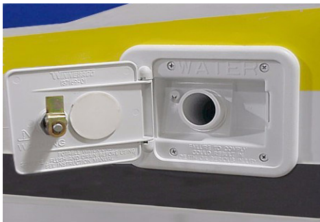
Water Tank Gravity Fill (typical)
