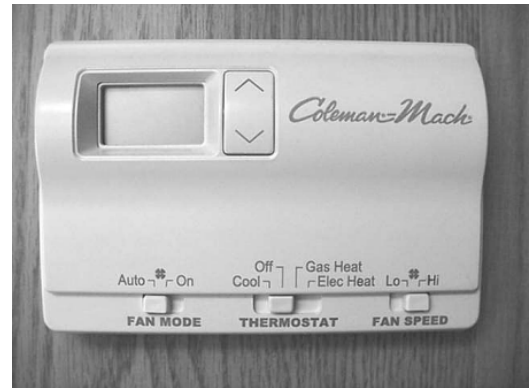
Gas Heat = Gas Furnace Electric Heat = Heat Pump Cool = Roof Air Conditioner
