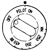
Oven Control Knob in "PILOT ON" position
